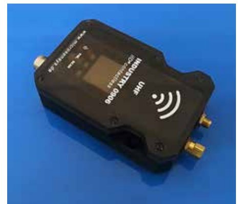
iID®INDUSTRY0906 – RFID reader module with integrated or external antenna option
