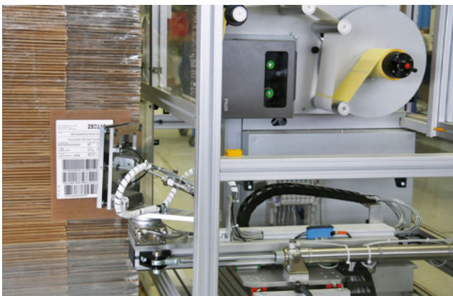
Applying labels to stacks of corrugated cardboard
