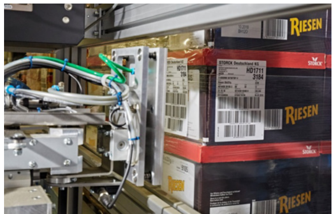
Double-sided labeling on the longitudinal and back sides
