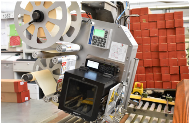
Print and apply system for wrap-around labeling
